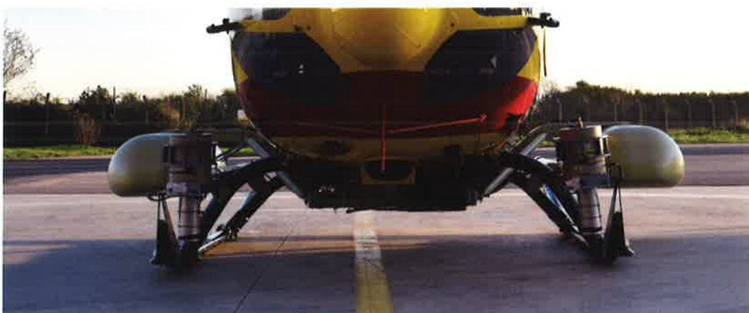
Symetrical assembly of detectors in the cradle installed under the helicopter
