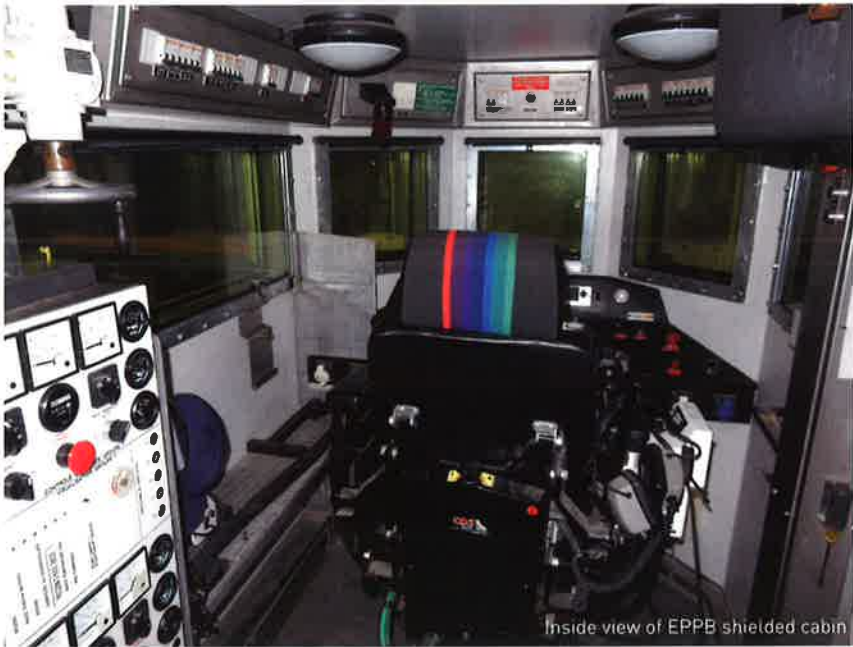
Shielded control station with support systems : nuclear ventilation system and power generator
