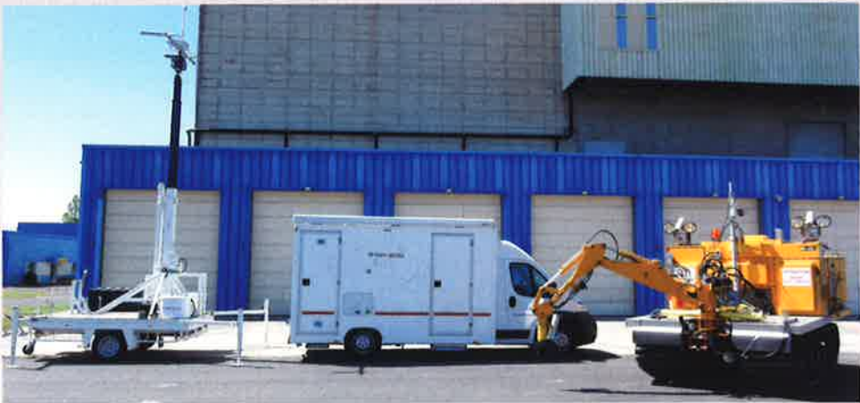
Outdoor equipment suite: antennas mast trailer, control station and ERASE
