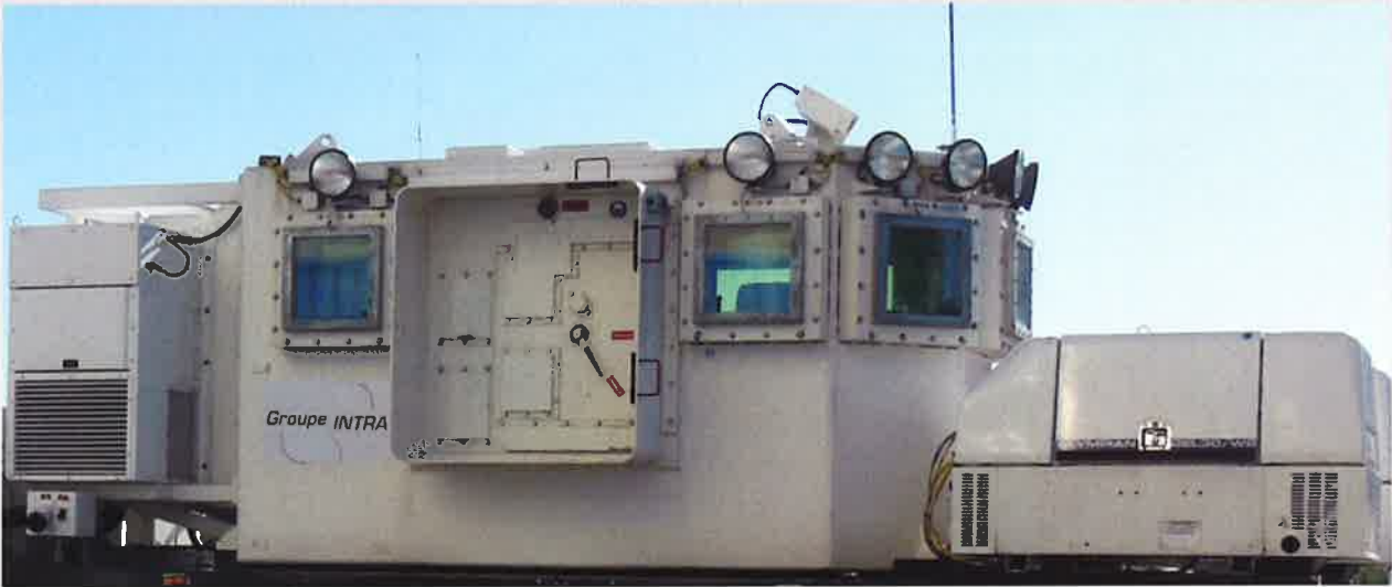
Shielded control station with support systems : nuclear ventilation system and power generator
