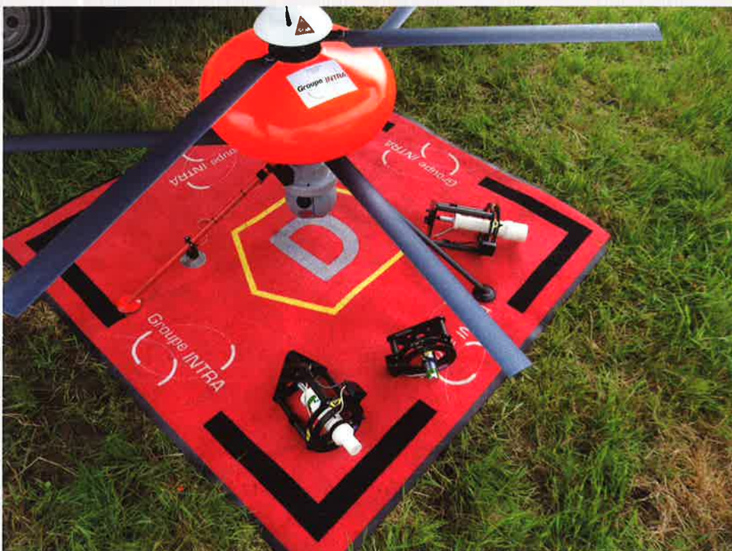
Electric UAV with battery, ball camera and radiological detector.
